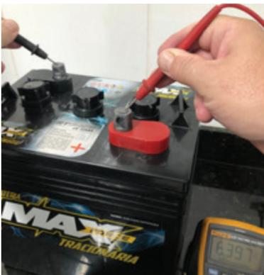
**Measuring mode with multimeter**
